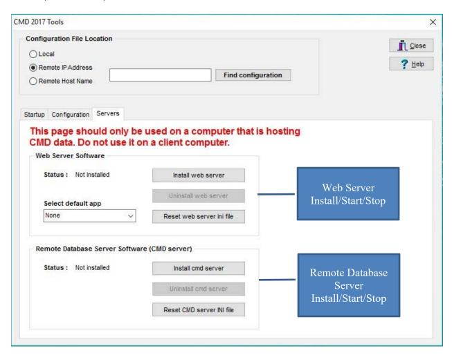
In the screen grab above, there are two group boxes, one to control the Web Server software, and the lower one, to control the Remote Database Server software. Note that in the screen grab above, neither of the servers are installed and running.
